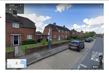
At both locations, replace the existing pole and flag with a battery operated RTPI on new post (mounted at the top of the pole like a bus stop flag)
